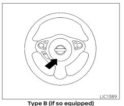
To sound the horn, push near the horn icon on the steering wheel.
