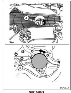
3. Place a large drain pan under the oil filter **B**.
