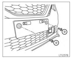
Type B (if so equipped) Type B (if so equipped) without grommets: Install the license plate bracket to the front bumper fascia using the two screws (**D**) provided.
