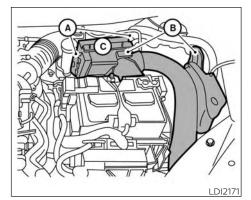
The air cleaner filter should not be cleaned and reused. Replace it according to the maintenance log shown in the "Maintenance and schedules" section of this manual
