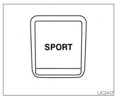
The SPORT mode switch adjusts the throttle sensitivity and transmission points to enhance performance. Push the SPORT mode switch on the instrument panel to activate. The SPORT mode indicator light (on the speedometer) will illuminate. The SPORT mode indicator light will remain lit while the mode is active
