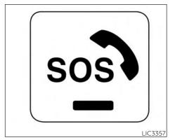
The E-call (SOS) switch is used in combination with a NissanConnect® Services subscription to call for assistance in case of an emergency.
