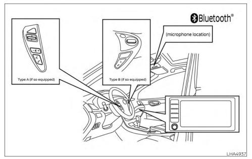
Your NISSAN is equipped with the Bluetooth® Hands-Free Phone System. If vou have a compatible Bluetooth® enabled cellular phone, you can set up the wireless connection between your cellular phone and the in-vehicle phone module. With Bluetooth® wireless technology, you can make or receive a hands-free telephone call with your cellular phone in the vehicle.
