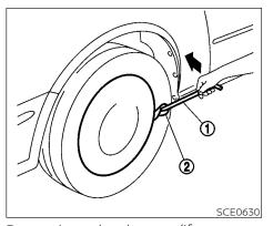
Removing wheel cover (if so equipped)
