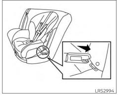
Forward-facing rigid-mounted - step 2 seating positions that do not have a top tether anchor.
