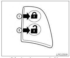
**Driver's and passenger's side**LOCKING WITH POWER DOOR
