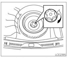
3. Turn the clamp counterclockwise and remove to release the spare tire.
