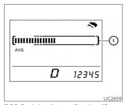
ECO Pedal Indicator Display (if so equipped)
