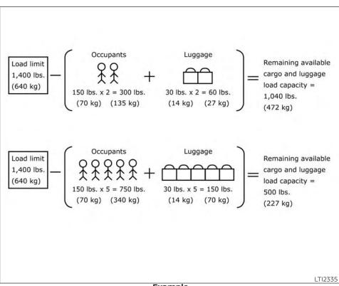
Steps for determining correct load limit
