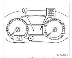
Type A (if so equipped) LOOSE FUEL CAP warning
