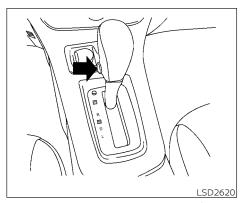
Overdrive (O/D) OFF switch (if so equipped)
